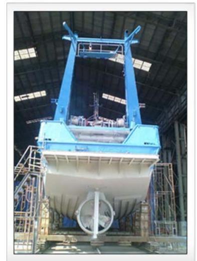
Ocean searcher Stern showing DuckBoard and rear deck access for hoisting material onboard using the H frame and deck winches
